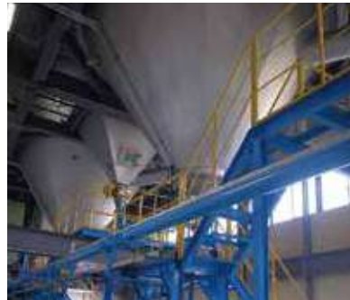
Atomization mode: Rotary atomizer Drying chamber diameter: \phi 5000 mm Liquid material processing capacity: 350 kg/h
