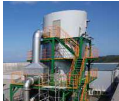
Atomization mode: Rotary atomizer Drying chamber diameter: \phi 5000 mm Liquid material processing capacity: 500 kg/h
