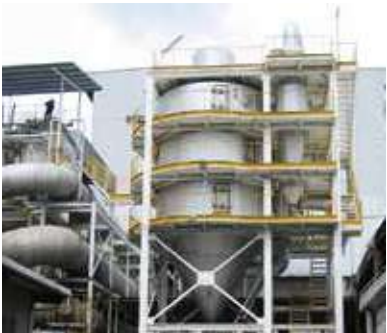
Atomization mode: Pressure nozzle Drying chamber diameter: \phi 4800 mm Water evaporation capacity: 1200 kg/h
