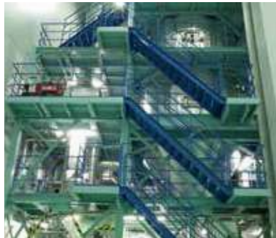
Atomization mode: Rotary atomizer Drying chamber diameter: \phi 4000 mm Water evaporation capacity: 100 kg/h
